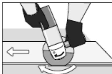
Otherwise, the danger exists of it being pushed uncontrollably out of the cut.
